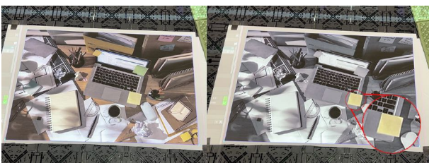
Fig 2: Colorization on the part of the printed image: (left) color projection on monochrome print (right) selective color projection on monochrome print with highlighting on post-note with yellow
