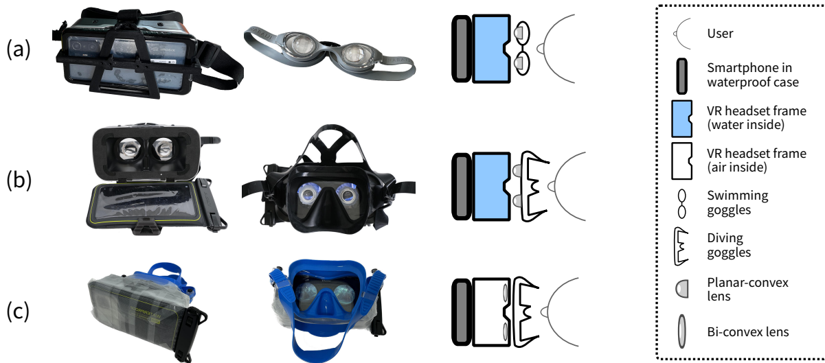
Fig. 1: Comparison of underwater VR HMD prototypes: (a) Prototype 1, (b) Prototype 2, and (c) Prototype 3, showcasing water-permeable and waterproof design ideas. Note: Prototype 3, initially designed as waterproof, experienced minor leakage with a small amount of water entering the HMD, but without impacting the visual quality of the VR experience.
