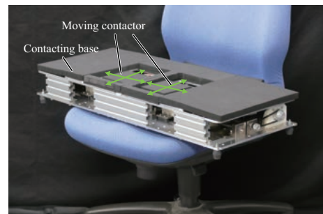
図 1: The 2-DoF buttock skin stretch device
