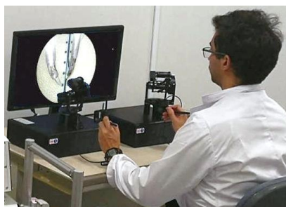
Figure 6: VR simulation at the maximum level of difficulty being operated by using haptic interfaces.
