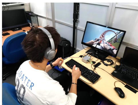
図 1: Procedure. Participant watches a video while holding a vibrator on each hand. Pink noise was played throughout the experiment.
