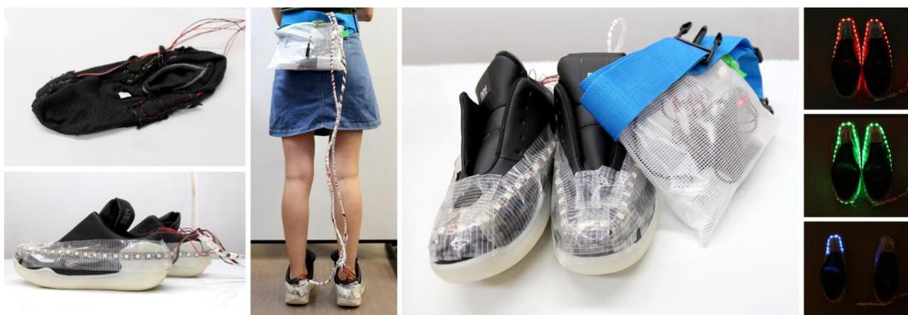
Figure 1: Left and central: The wearable prototype, including haptic-enabled socks and Orphe shoes with LED lights. Right: The expert-receiver system featuring the visual modality. From top to bottom: Wrong action (Mode 2), Right action (Mode 2), Move the left foot to the north (Mode 1).
